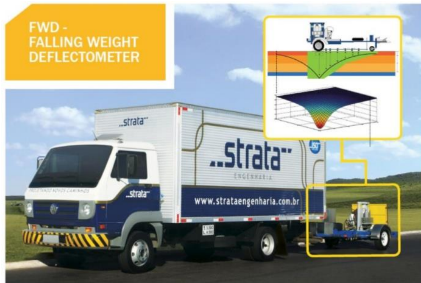
Figura 2 – FWD: Falling Weight Deflectometer
